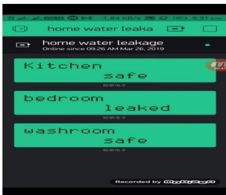
Fig 10. Result when leakage detected in Bedroom pipe
